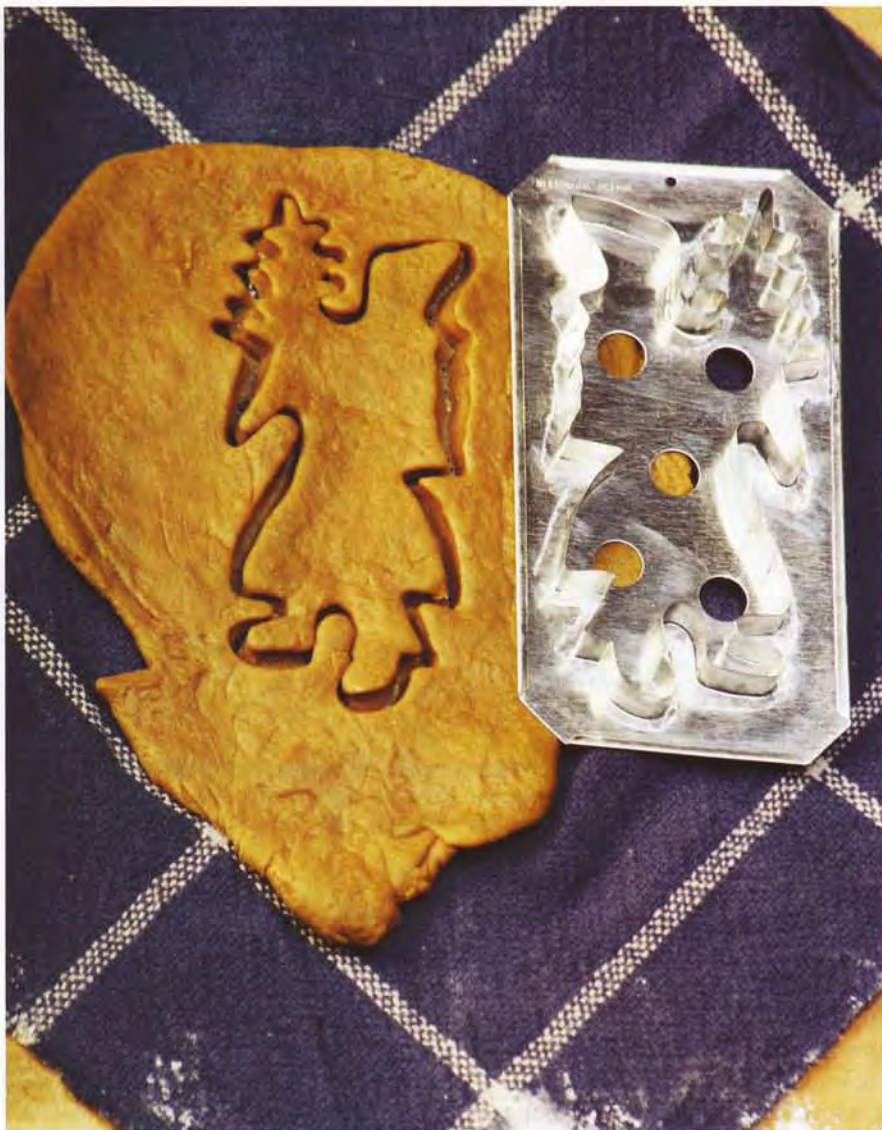
At the Victor Trading Company, Karen Morrison creates thousands of cookie cutters in the basic manner of bending tin to match the line on a pattern and then soldering the strip to a back piece. The Belsnickel above is a historic design, the cyclist is modern.
